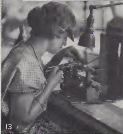
10—Piercing vent and stamping name on gold pen—dial feed press. 11—General view of gold pen slitting department. 12—Curving gold pen on forming press. 13—Cutting slit in gold pen. 14—General view of gold pen grinders.
